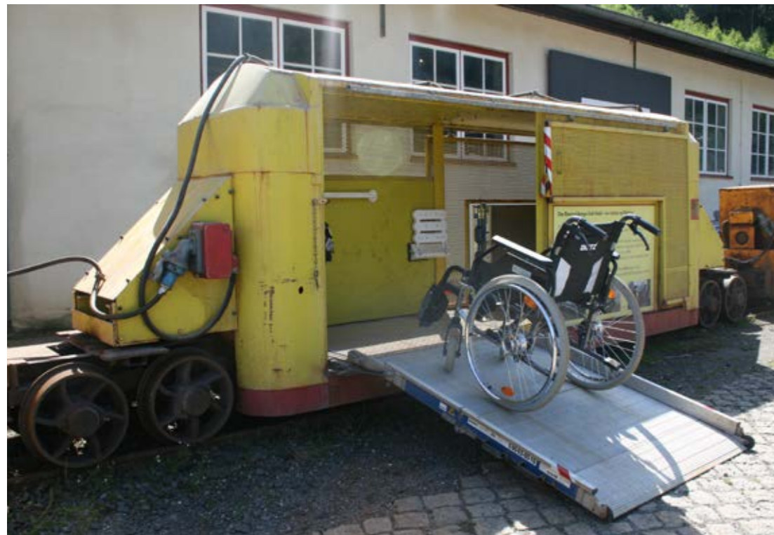
Figure 7: The converted mining car ©Weltkulturerbe Erzbergwerk Rammelsberg Goslar GmbH
